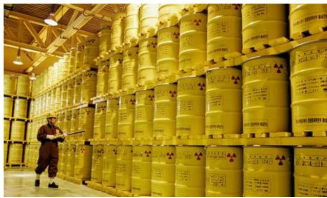
Industries and scientific establishments utilize radioactive sources for a wide range of applications. When the radioactive sources used by industry no longer emit enough penetrating radiation for them to be of use, they are treated as radioactive waste. Sources used in industry are generally short-lived and any waste
