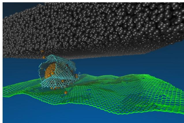
Graphene can also be used to better protect ball bearings, which can corrode over time when exposed to water, the process commonly referred to as tribo-corrosion. The Argonne-developed process based on graphene has shown that a few layers of graphene not only
