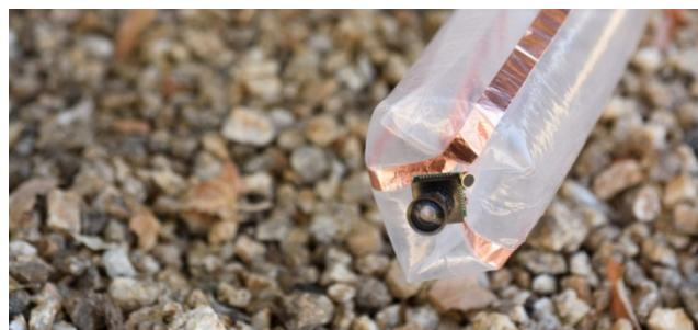
This is just one possible application of a new type of robot created by mechanical engineers at Stanford University, detailed in a recent *Science Robotics* [paper](#). Inspired by natural organisms that cover distance by growing – such as vines, fungi and nerve cells – the researchers have made a proof of concept of their soft, growing robot and have run it through some challenging tests.
