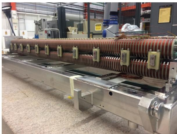
One of the Argonne projects was the design and construction of the LCLS-I undulator system – 440 feet of sophisticated technical components that incorporated 33 cutting-edge undulators. The LCLS-I facility at the SLAC National Accelerator Laboratory has now been operating successfully for more than seven years.
