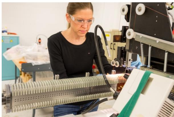
“The main challenge is to maintain the consistent wiggle motion of electrons inside of an SCU,” said Gluskin, adding that the range of accepted deviation from the straight line of the beam motion across the distance of several meters is just a few microns. For comparison, an average human hair is 100 microns wide.
