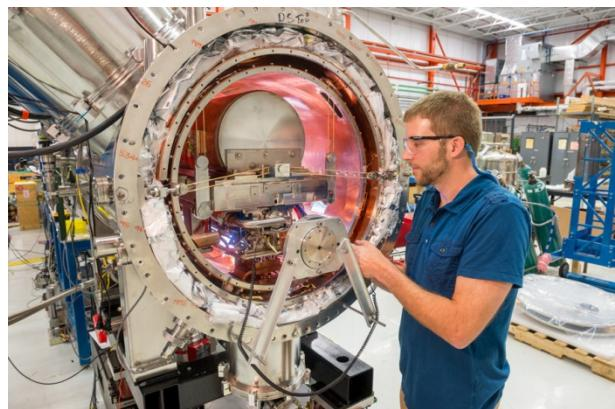
The team at the Department of Energy's Advanced Photon Source (APS) at Argonne successfully built and tested a 1.5-meter-long prototype SCU magnet designed to meet FEL undulator requirements. This SCU utilizes niobium-titanium superconducting wire for winding its magnetic coils.
