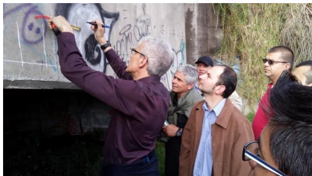
Practical session on the structure of the bridge over the Rumiñahui River. Demonstration of the methodology to follow while using the Schmidt sclerometer. (Photo: Eduardo Fco. Robles Piedras/ININ)
