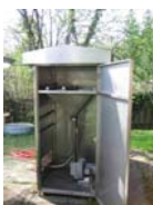
Aerosol Sampler 88 Nm 3 /h Glass microfiber filter GF/A
